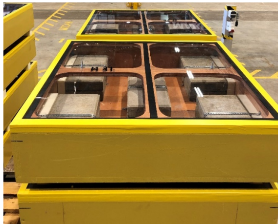
Figure 2-4: Photo of exemplary modules with fix ballasts inside the hull (left) and additional ones on deck for trimming (right)
