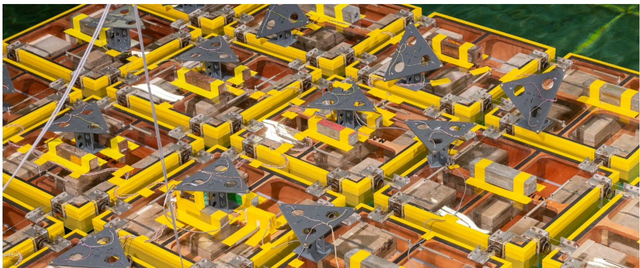
Figure 4-3: Triangular position targets on selected modules for contact-less optical position measurement system
