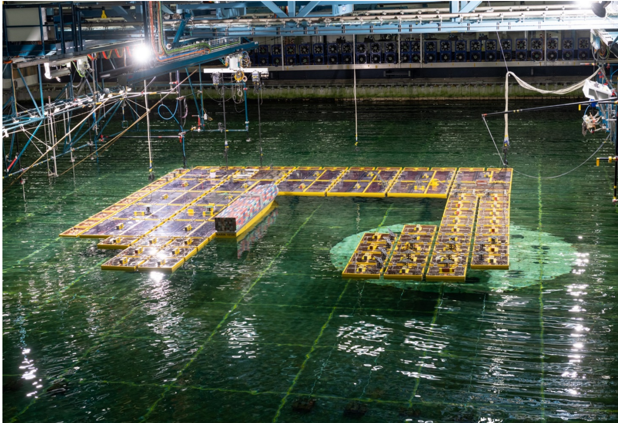
Figure 2-2: Modelsetup of Space@Sea island in MARIN's Offshore Basin
