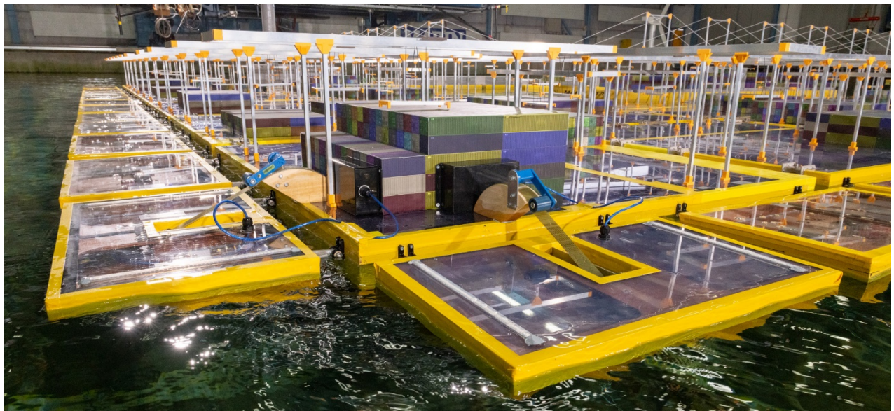
Figure 7-4: Photo of the modelled WECs including power take off system
